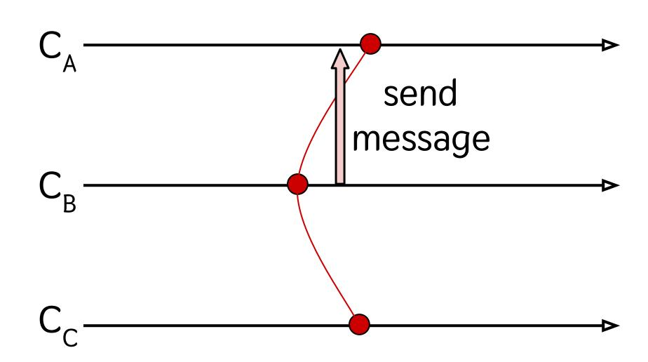
Inconsistent checkpoint: a message has been received by a process  $[C_A]$  but was never sent by the corresponding sender  $[C_B]$  (breaks normal sequence of events)
